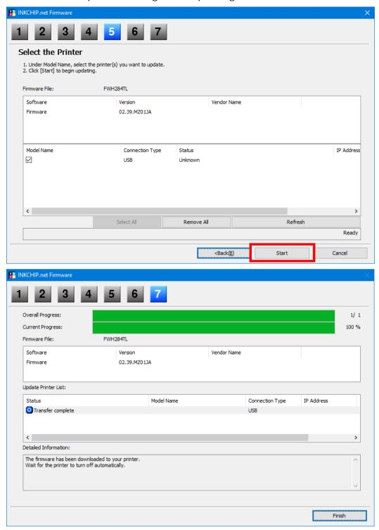
At this point, chipless firmware will be downloaded to the printer. The completion of the download process on to the printer will be indicated by the word "FINISHED" on the printer display. After that, press the "OK" button on the control panel and the printer will turn off.
